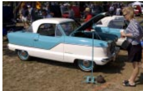
A 1959 Nash Metropolitan. It has a top speed of 78mph and an engine that puts out 52HP. Price when new: $1,774.60.
