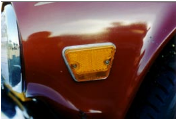
The correct lens for any car sold in America has a "bumpy" pattern on the upper \frac{3}{4} and horizontal lines at the bottom. The photo above shows a correct U.S. lens.
