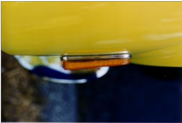
Correctly installed left side marker lens: When viewed from above, the thicker part of the lens goes towards the front of the car. This compensates for the inward curve of the fender near the headlight and keeps the side of the lens, the reflective portion, parallel with the side of the car.
