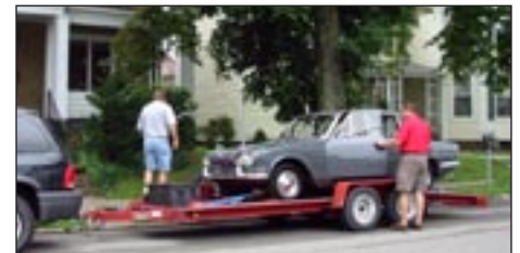
This LBC is in the process of being secured to the deck of this open flat-bed trailer. This trailer uses removable, adjustable wheel ramps to aid in loading of the LBC onto the trailer.
