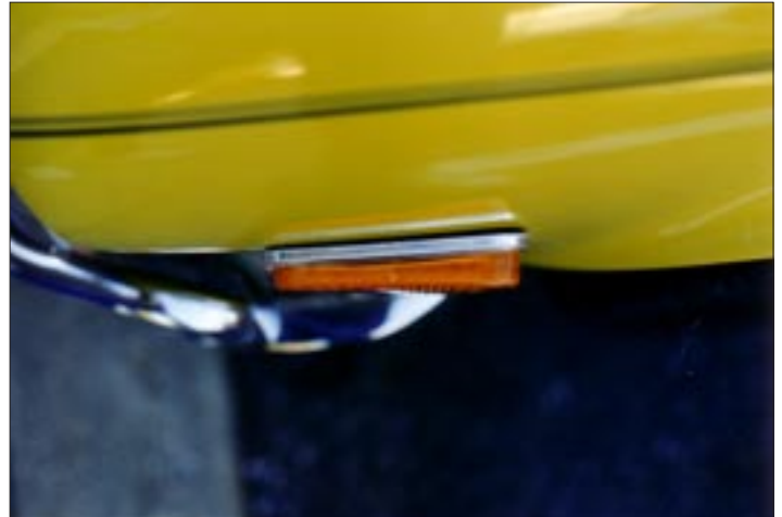
Incorrectly installed left hand side marker: note the thick part of the lens to the rear.
