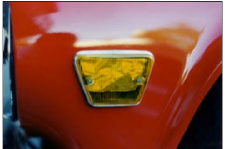
The U.K. spec lens has vertical lines across the entire lens and is quite clear, permitting a good view of the foil reflector behind the lens.
